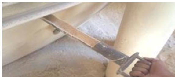
Figure 5: Sample Collection from Pre-Preheater Scale (LCP)
