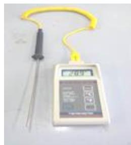
Figure 2: Thermometer to measure the temperature in cyclones
