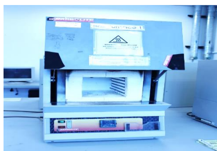
Figure 4: Scientific ISO-temp Programmable Muffle Furnace
