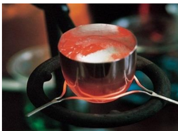
Figure (6): Sample preparation in platinum crucible
