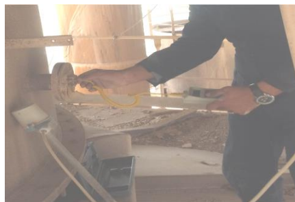
Figure 3: Taking readings from the thermocouple apertures
