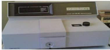
Figure (2) Spectrophotometer apparatus for Measurement of concentration cupper
