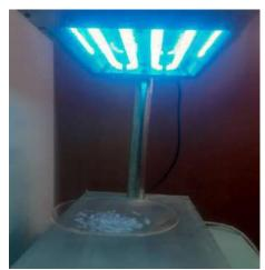
Figure(3) exposure sample from plastic straw to UV energy at t=5 hr.
